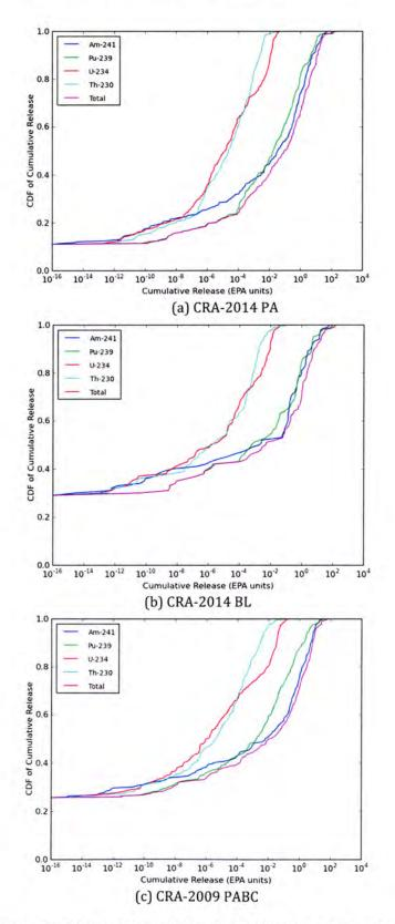
Figure 3 Normalized cumulative release (EPA units) to the Culebra from the borehole for each isotope and the total for an E1 intrusion at 350 years: (a) CRA-2014 PA, (b) CRA-2014 BL, and (c) CRA-2009 PABC.
