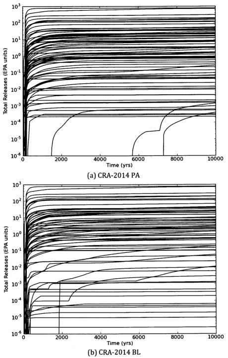
**Figure 26(a,b)** Cumulative total releases to the Culebra for an E2-E1 intrusion at 100 years in the (a) CRA-2014 PA, (b) CRA-2014 BL, and (c) CRA-2009 PABC.
