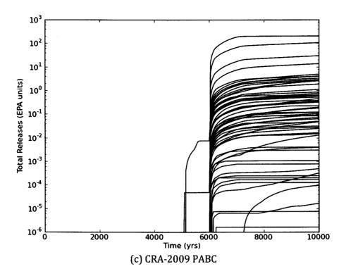
**Figure 30(c)** Cumulative total releases to the Culebra for an E2-E1 intrusion at 6000 years in the (a) CRA-2014 PA, (b) CRA-2014 BL, and (c) CRA-2009 PABC.
