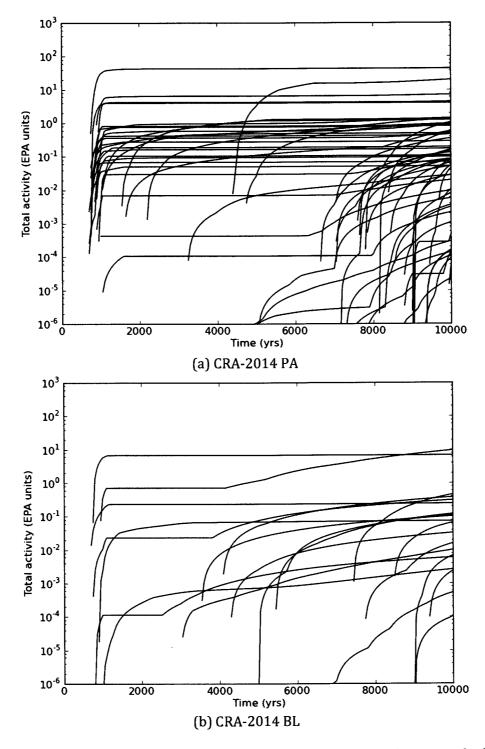
**Figure 20(a,b)** Cumulative total releases to the Culebra for an E2 intrusion at 350 years in the (a) CRA-2014 PA, (b) CRA-2014 BL, and (c) CRA-2009 PABC.
