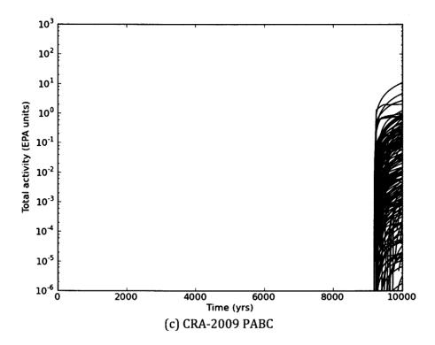
**Figure 18(c)** Cumulative total releases to the Culebra for an E1 intrusion at 9000 years in the (a) CRA-2014 PA, (b) CRA-2014 BL, and (c) CRA-2009 PABC.
