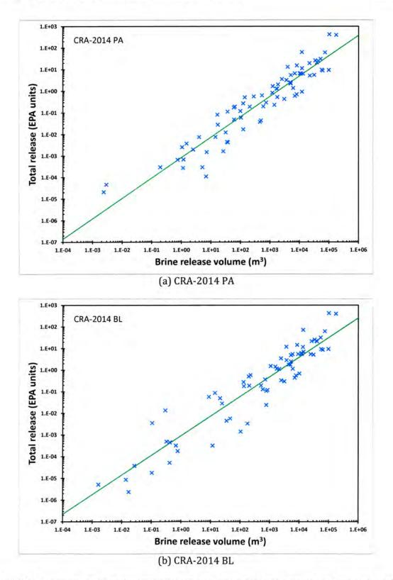
Figure 10(a,b) Sensitivity analysis for total releases as a function of brine release volume in the (a) CRA-2014 PA, (b) CRA-2014 BL, and (c) CRA-2009 PABC.
