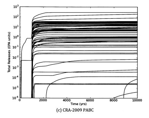
**Figure 28(c)** Cumulative total releases to the Culebra for an E2-E1 intrusion at 1000 years in the (a) CRA-2014 PA, (b) CRA-2014 BL, and (c) CRA-2009 PABC.
