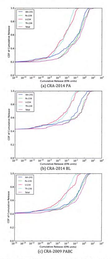
**Figure 4** Normalized cumulative release (EPA units) to the Culebra from the borehole for each isotope and the total for an E1 intrusion at 1000 years; (a) CRA-2014 PA, (b) CRA-2014 BL, and (c) CRA-2009 PABC.
