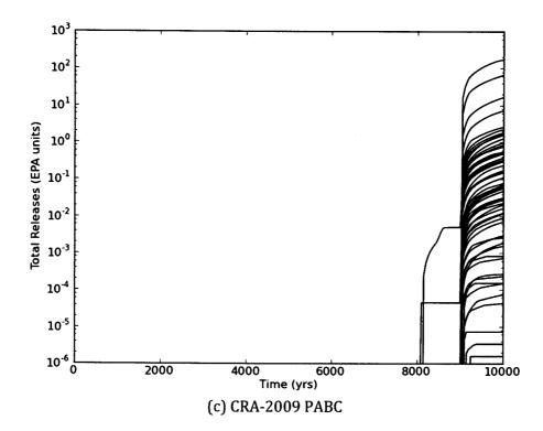
**Figure 31(c)** Cumulative total releases to the Culebra for an E2-E1 intrusion at 9000 years in the (a) CRA-2014 PA, (b) CRA-2014 BL, and (c) CRA-2009 PABC.
