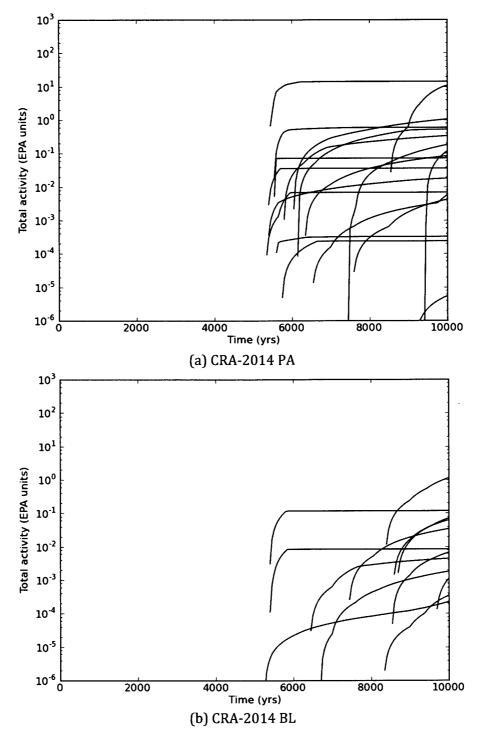
**Figure 23(a,b)** Cumulative total releases to the Culebra for an E2 intrusion at 5000 years in the (a) CRA-2014 PA, (b) CRA-2014 BL, and (c) CRA-2009 PABC.
