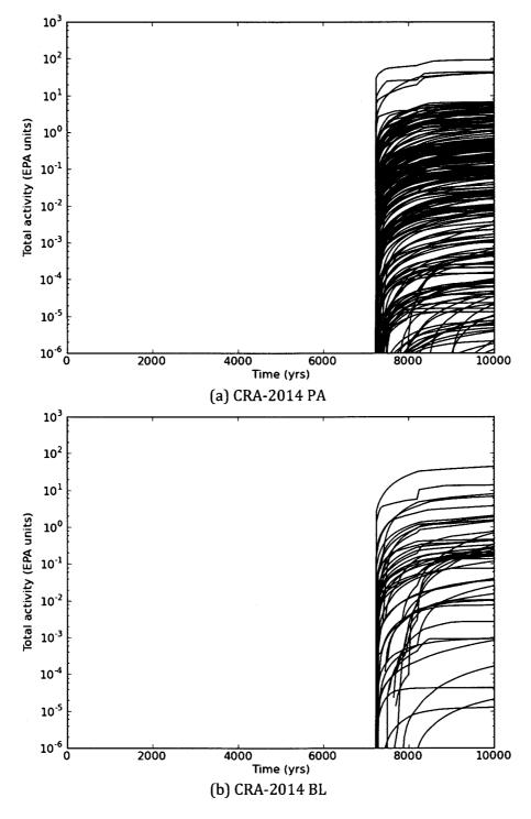
**Figure 17(a,b)** Cumulative total releases to the Culebra for an E1 intrusion at 7000 years in the (a) CRA-2014 PA, (b) CRA-2014 BL, and (c) CRA-2009 PABC.
