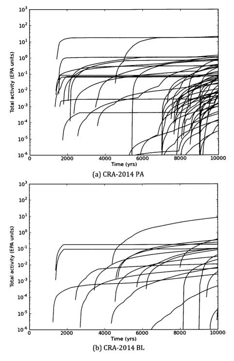
**Figure 21(a,b)** Cumulative total releases to the Culebra for an E2 intrusion at 1000 years in the (a) CRA-2014 PA, (b) CRA-2014 BL, and (c) CRA-2009 PABC.
