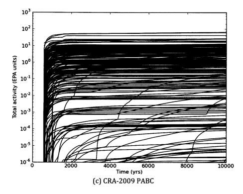
**Figure 13(c)** Cumulative total releases to the Culebra for an E1 intrusion at 350 years in the (a) CRA-2014 PA, (b) CRA-2014 BL, and (c) CRA-2009 PABC.
