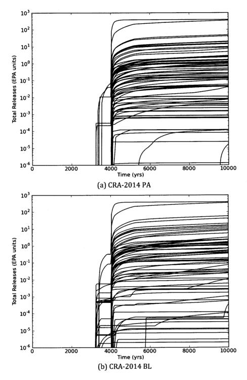
**Figure 29(a,b)** Cumulative total releases to the Culebra for an E2-E1 intrusion at 4000 years in the (a) CRA-2014 PA, (b) CRA-2014 BL, and (c) CRA-2009 PABC.
