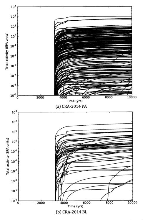
**Figure 15(a,b)** Cumulative total releases to the Culebra for an E1 intrusion at 3000 years in the (a) CRA-2014 PA, (b) CRA-2014 BL, and (c) CRA-2009 PABC.
