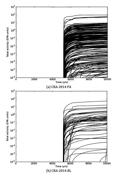
**Figure 16(a,b)** Cumulative total releases to the Culebra for an E1 intrusion at 5000 years in the (a) CRA-2014 PA, (b) CRA-2014 BL, and (c) CRA-2009 PABC.
