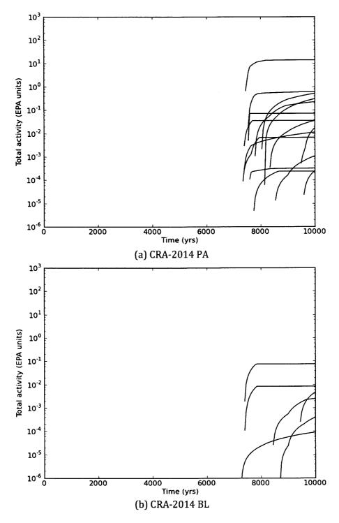
**Figure 24(a,b)** Cumulative total releases to the Culebra for an E2 intrusion at 7000 years in the (a) CRA-2014 PA, (b) CRA-2014 BL, and (c) CRA-2009 PABC.
