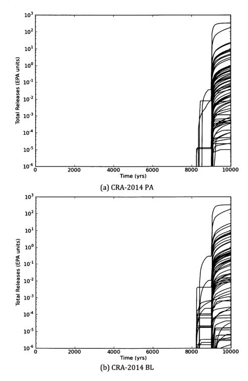
**Figure 31(a,b)** Cumulative total releases to the Culebra for an E2-E1 intrusion at 9000 years in the (a) CRA-2014 PA, (b) CRA-2014 BL, and (c) CRA-2009 PABC.
