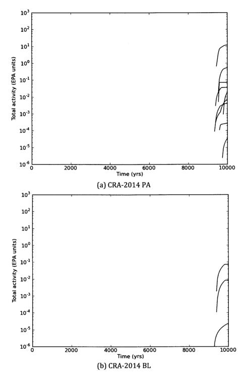
**Figure 25(a,b)** Cumulative total releases to the Culebra for an E2 intrusion at 9000 years in the (a) CRA-2014 PA, (b) CRA-2014 BL, and (c) CRA-2009 PABC.
