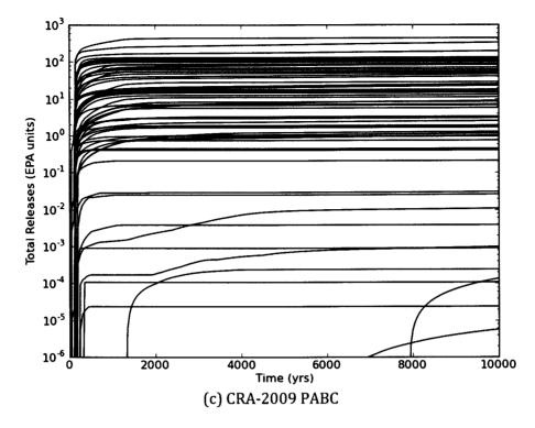
**Figure 26(c)** Cumulative total releases to the Culebra for an E2-E1 intrusion at 100 years in the (a) CRA-2014 PA, (b) CRA-2014 BL, and (c) CRA-2009 PABC.
