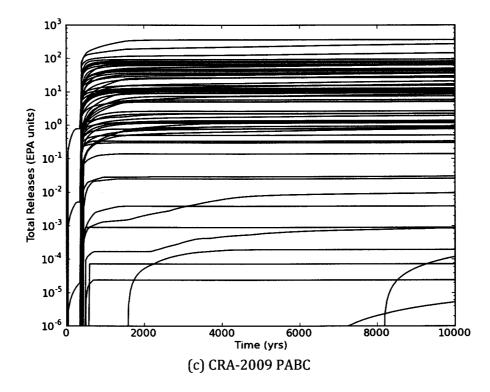
**Figure 27(c)** Cumulative total releases to the Culebra for an E2-E1 intrusion at 350 years in the (a) CRA-2014 PA, (b) CRA-2014 BL, and (c) CRA-2009 PABC.
