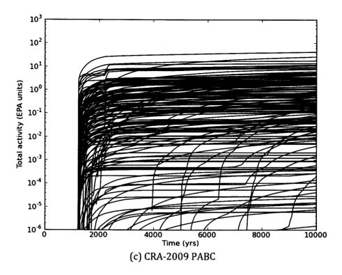
**Figure 14(c)** Cumulative total releases to the Culebra for an E1 intrusion at 1000 years in the (a) CRA-2014 PA, (b) CRA-2014 BL, and (c) CRA-2009 PABC.
