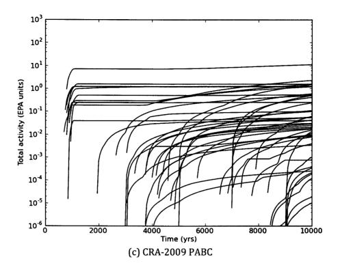
**Figure 20(c)** Cumulative total releases to the Culebra for an E2 intrusion at 350 years in the (a) CRA-2014 PA, (b) CRA-2014 BL, and (c) CRA-2009 PABC.
