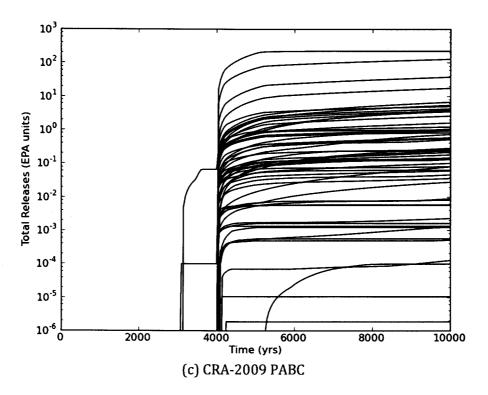
**Figure 29(c)** Cumulative total releases to the Culebra for an E2-E1 intrusion at 4000 years in the (a) CRA-2014 PA, (b) CRA-2014 BL, and (c) CRA-2009 PABC.
