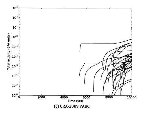
**Figure 23(c)** Cumulative total releases to the Culebra for an E2 intrusion at 5000 years in the (a) CRA-2014 PA, (b) CRA-2014 BL, and (c) CRA-2009 PABC.
